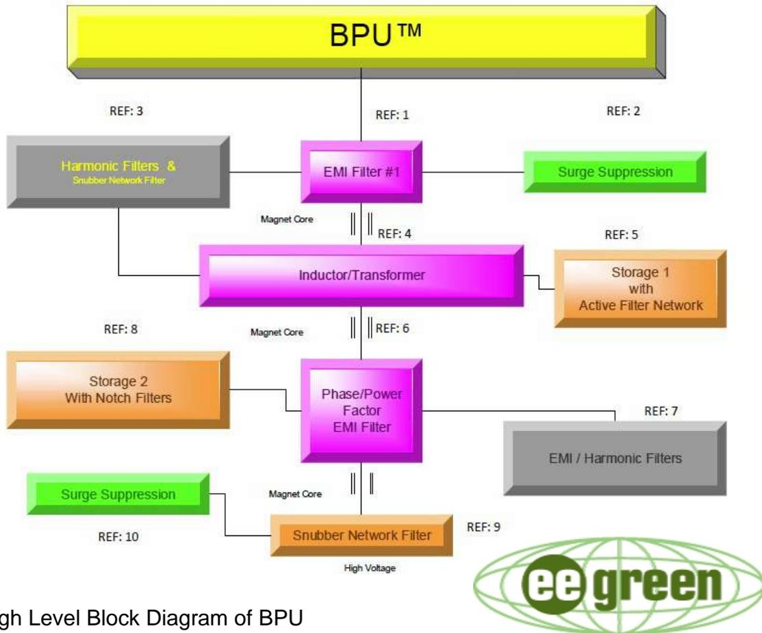
High Level Block Diagram of BPU
